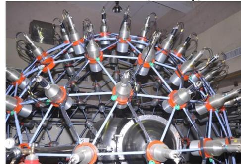
**National Array of Neutron Detectors (NAND)** is an array of 100 liquid-scintillator based neutron detectors which is used to study fission dynamics through pre- and post- fission neutron multiplicities using beams delivered by Pelletron-LINAC at IUAC. This is one of a few large neutron detector arrays in the world.
