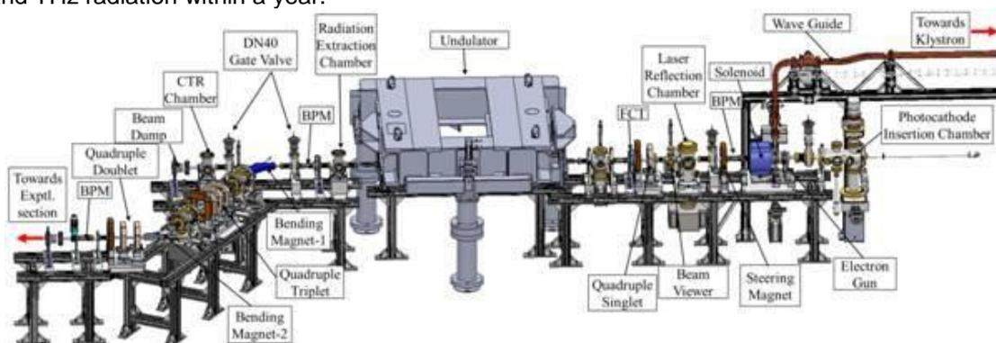
The design of the complete beam line of the Free Electron Laser facility
