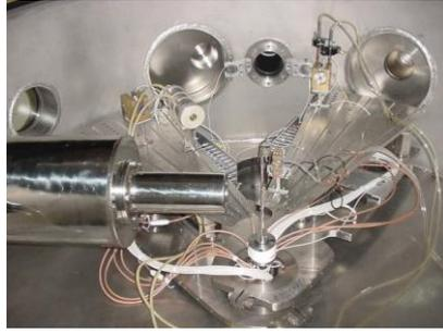
**General Purpose Scattering Chamber (GPSC)** is being extensively used for both nuclear physics as well as materials science experiments (e.g. the studies of Heavy Ion scattering and transfer reactions above barrier, Projectile Breakup and for ion irradiation).
