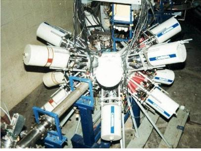
**Gamma Detector Array (GDA)**, consists of 12 Compton suppressed, HPGe detector setup, which was later augmented with a recoil distance based lifetime measuring plunger equipment, a charge particle detector array and an electromagnet for perturbed angular correlation measurement studies.
