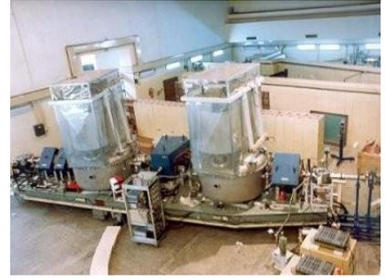
**Heavy Ion Reaction Analyzer (HIRA)** is one of the few Recoil Mass Spectrometers (RMS) in the world and the first of its kind in Asia. HIRA facilitates the study of heavy ion induced nuclear reaction dynamics, operates in the direction of primary beam, separates ions of various masses and has provided India's first RIB, namely,  ${}^7\text{Be}$ .
