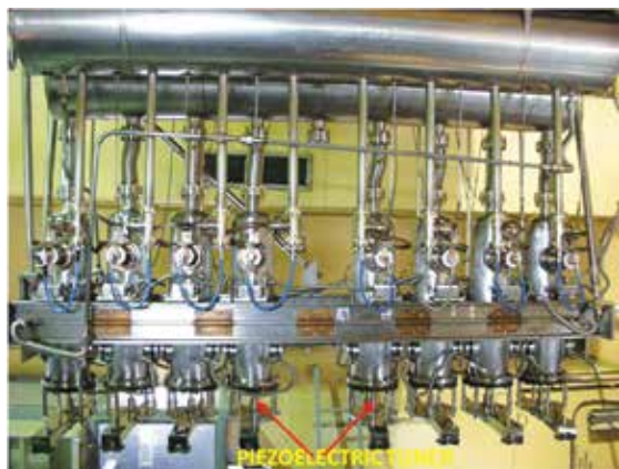
Fig. 1. LINAC cryostat with piezoelectric tuners.
