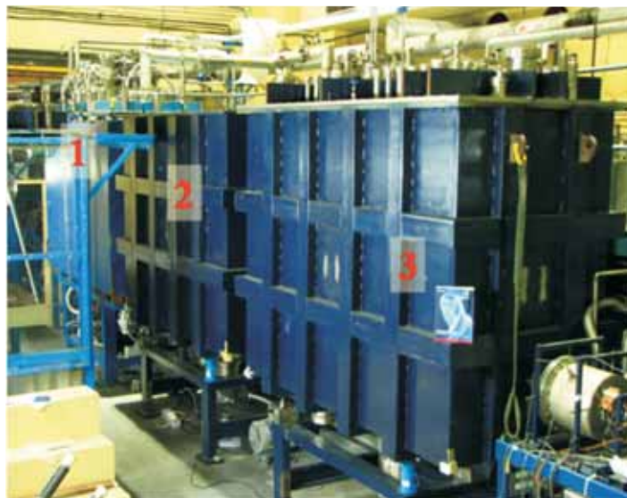
Fig. 2. The remaining cryostats 2 and 3 installed in the beam line
