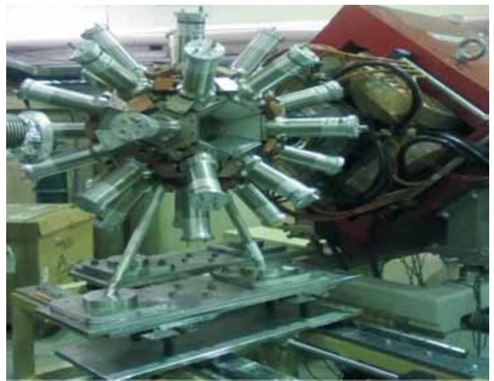
Fig.1. 4\pi spin spectrometer at HYRA target site on specially made structure
