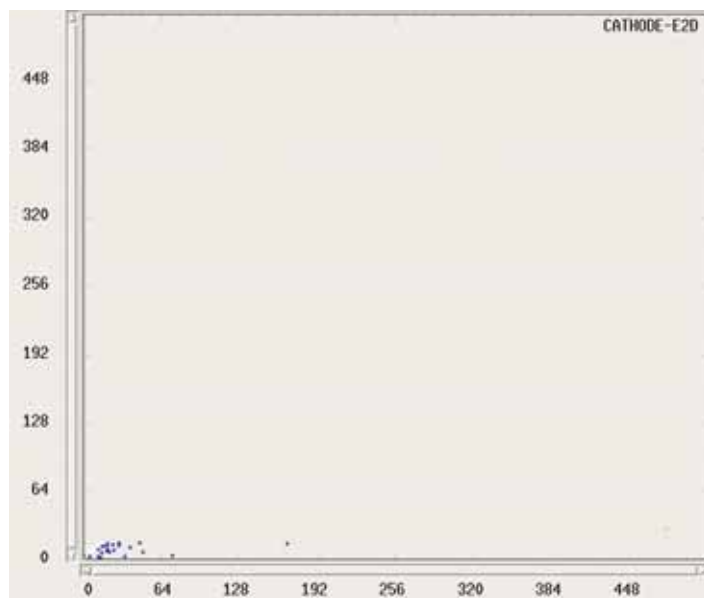
Fig. 1b Energy loss versus total energy for ^{48}\text{Ti} on ^{27}\text{Al} but with HYRA set as in Fig. 1a; Focal plane is free from beam background
