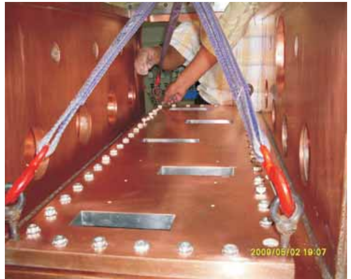
Fig. 1. Copper plated prototype RFQ chamber
