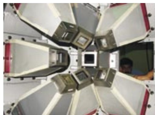
Fig.11: The inside view of INGA during installation in Beam hall II
