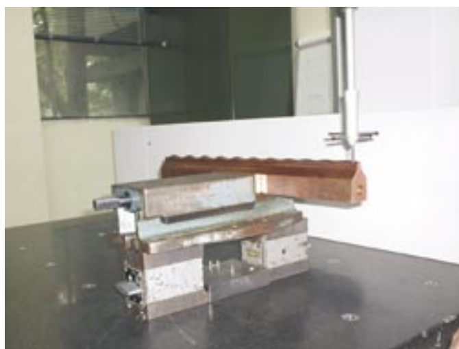
Fig.2. Modulated vanes being tested for dimensional accuracy.
