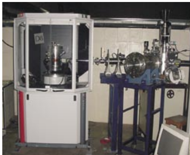
Fig.3. In-situ X-ray diffractometer at materials science beam line at beam hall-II.
