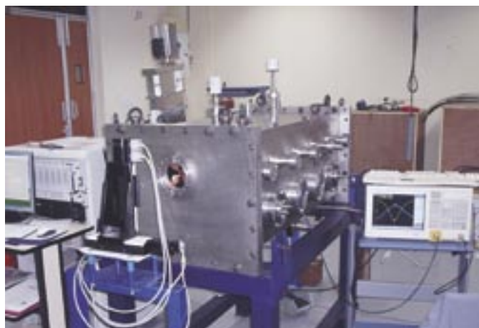
Fig.1. Bead pull apparatus and prototype RFQ
