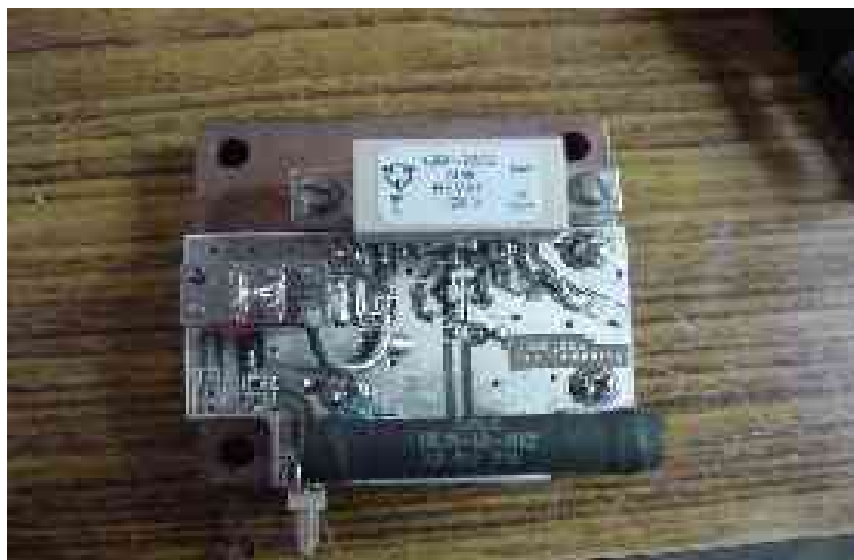
Fig: VHF Pre-Driver Amplifier
