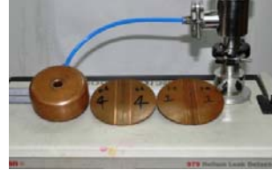
Figure 3: Laser-welded OFE copper samples.
