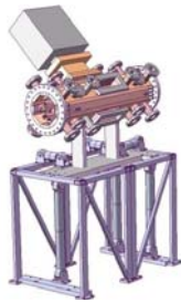
Figure 1: First module of LEHIPA RFQ with its support structure.
