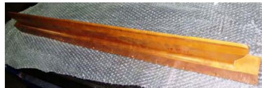
Figure 4: A 400 keV RFQ Minor Vane.
