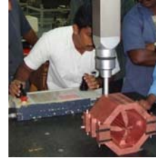
Figure 3: The CMM Inspection of RFQ cavity.
