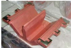
Figure 2: A short length major vane showing brazing arrangement.
