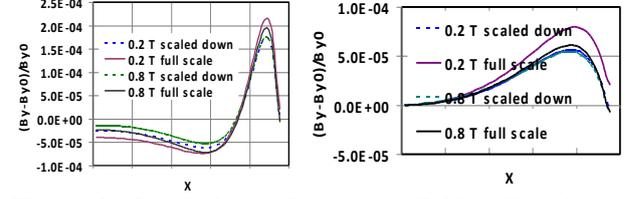
Figure 2: Comparison of magnetic field uniformities at the 1<sup>st</sup> quadrant of the upper boundary of the good field zone (left) and at the mid plane ( $y=0$ ) (right).
