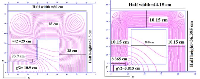
Figure 1: 1/4th cross-section of the full size (left) and scaled down dipole magnet (right) (all dimensions in cm).
