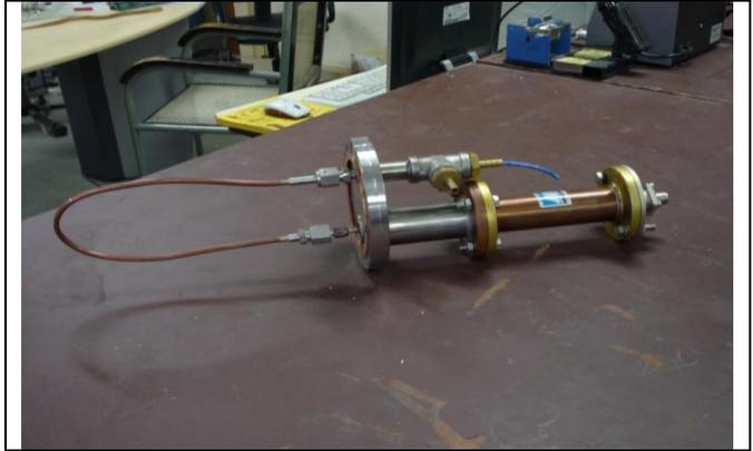
Figure 3: View of the Air cooled RF Coupler
