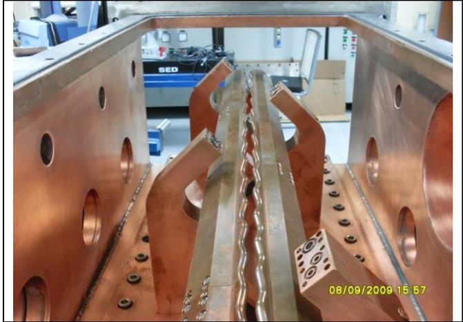
Figure 1: General assembly of the prototype of 1.17m modulated copper plated RFQ at IUAC.
