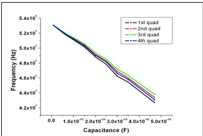
Figure 2: Frequency shift in capacitive variation method.
