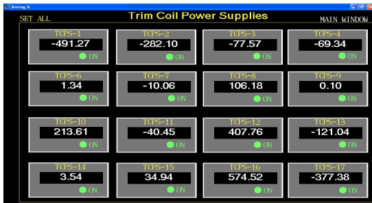
Figure 2: Trim Coil Power Supplies Interface.
