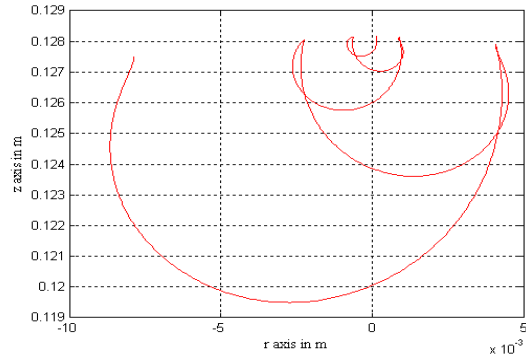
Figure 3: Trajectory of an electron at 18MV/m field.
