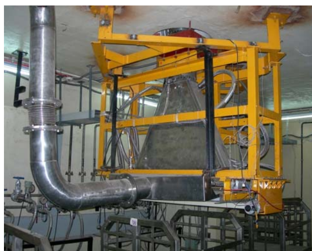
Figure 1: Linac Irradiation facility showing electron gun, RF Cavity at first floor and horn, conveyor etc. at ground floor.
