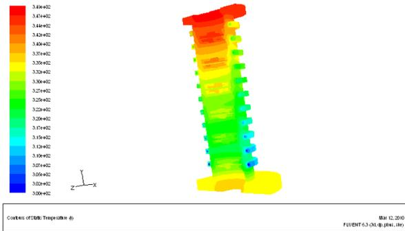
Figure 1: Temperature profile of operating LINAC.
