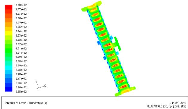
Figure 2: Temperature profile of new LINAC.
