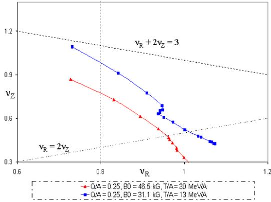
Figure 3: Tune diagram before extraction
