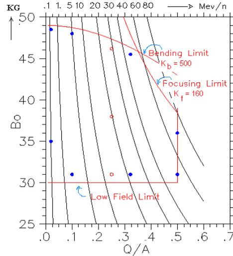
Figure 1: Operating diagram in  $(B_0, Q/A)$  plane
