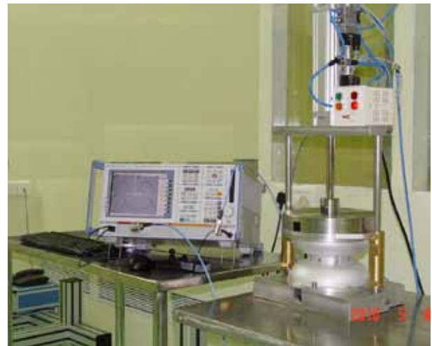
Fig. 1 :- RF Frequency measurement set up for 1.3GHz SCRF cavities
