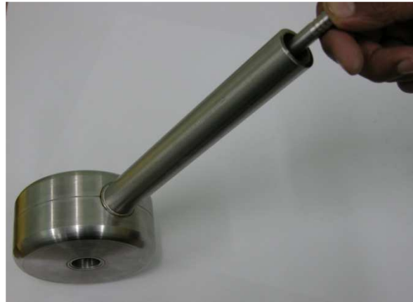
Figure 1: Laser Beam welded drift tube assembly with embedded PM Quadrupoles.
