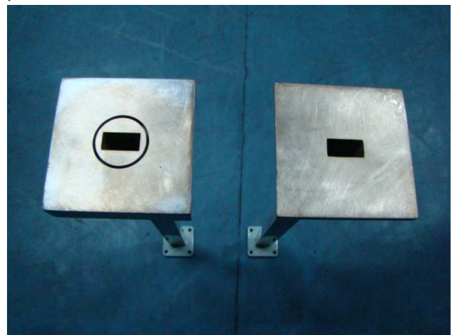
Figure 6: Choke and cover flange of waveguide break Microwave power was varied in steps of 10W and reflected power was within 1W for 200W transmitted power.
