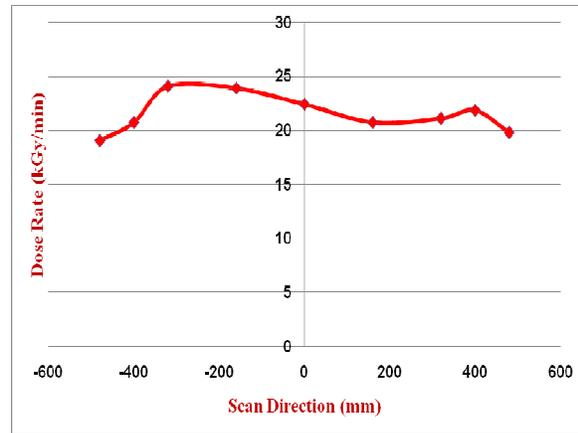
Figure 4: Dosimetric Profile of Electron Beam
