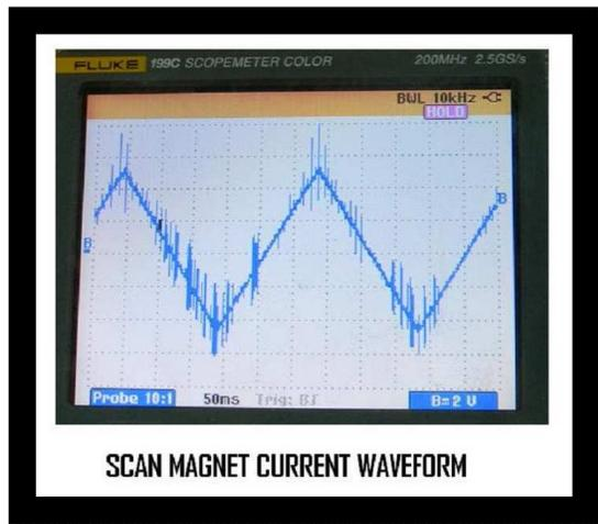
Figure 2: Current Waveform.
