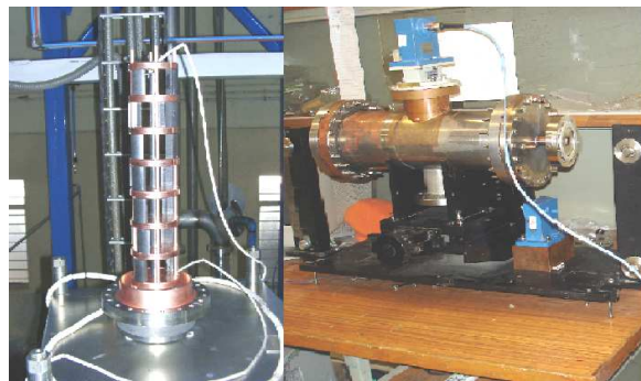
Figure 2: 8-cell PWT linac array and final assembly.
