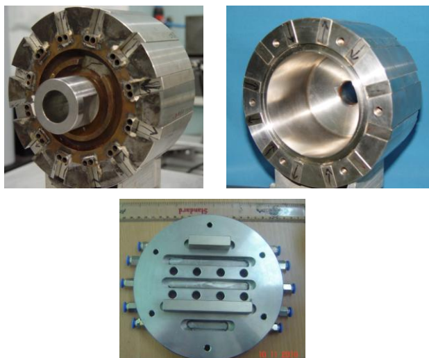
Fig.2 Plasma chamber fabricated in stainless-steel with arrangements of permanent magnets and cooling channels on the chamber and its side flange. Small cylindrical neck is provided for placement of filter magnets and coupling it with the ion extraction system.
