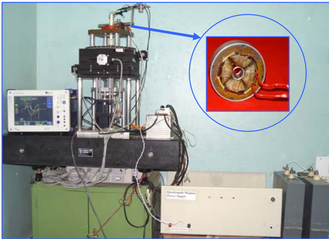
Figure 2: Quadrupole magnet pulse field measurement setup. Inset Quadrupole magnet
