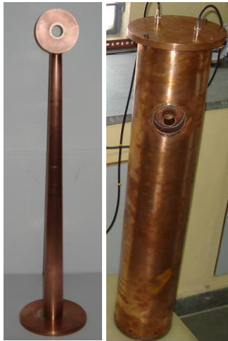
Figure 2: Copper model of the low beta resonator.
