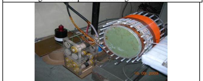
Fig. 5 Test tank circuit (110μH, 23nF) For gun power supply unit testing
