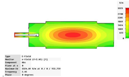
Fig 4: CST simulation of the coaxial-antenna coupling to the plasma chamber
