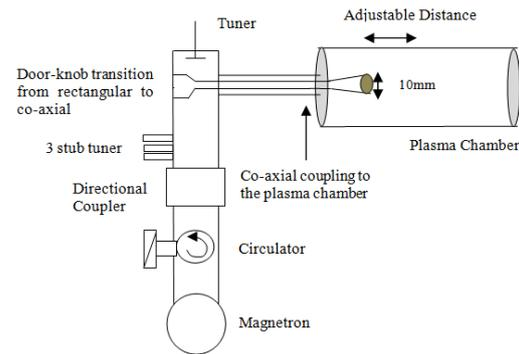
Fig 5: Schematic of the RF injection line of the ECRIS
