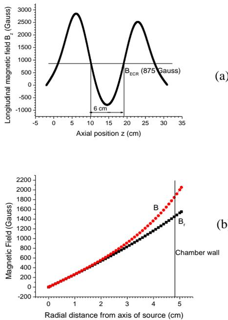
Fig 3: (a) Longitudinal component of magnetic field ( $B_z$ ) on the axis of the source. (b) Radial component ( $B_r$ ) and absolute value ( $B$ ) of magnetic field vs. radial position, at an axial distance of 3 cm from the centre of the source.
