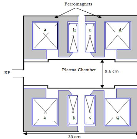
Fig 1: Coil Structure of the 2.45 GHz ECRIS. Direction of current for coils a & d is into of the plane of paper while it is reverse for coils b & c.
