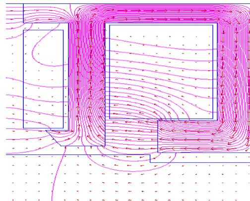
Fig 2 : POISSON simulation of magnetic field in one quarter of the source
